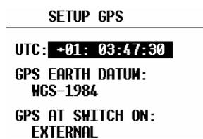
GPS earth datum is set to WGS 84 and not possible to be changed. GPS at switch on shows the status of GPS engine (internal or external) after switching on the unit. All necessary settings are done in the factory.
