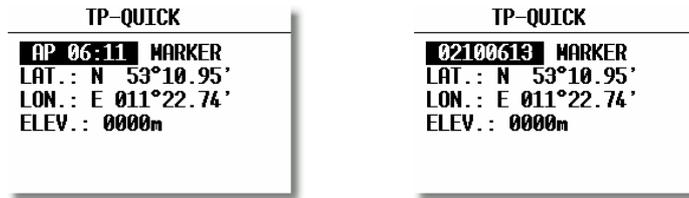
The names of such points are offered in two different forms. AP and TIME or date and time (02100613). The form depends on setting in setup after password (TP). All data can be edited immediately and stored. This procedure is useful to memorize convenient landing places, thermals etc...By default settings these points have MARKER attribute.
