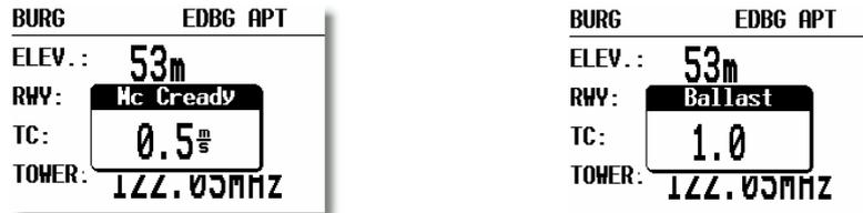
Second press on MC/Bal key will activate ballast input, use the same procedure like by MC.
