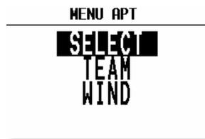
There are two ways to select an airport. The first direct way is using of ICAO code input. After code input the airport is selected.
