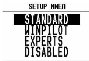
All NMEA sentences are not active in default setting, which means the pilot has to activate them if necessary. GGA and RMC are factory set (STANDARD). The pilots using Winpilot should **activate LXWP\_ also**. Experts will allow a bright spectrum of NMEA sentences.
